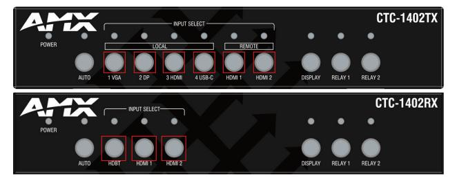
Press the AUTO Button (ensure AUTO LED is off) or the specific input button (in red frames above) to enable Manual Switching. In Manual Switching mode:
