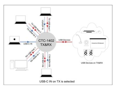
When the USB-C input is selected, the USB devices can be connected to the PC directly.
