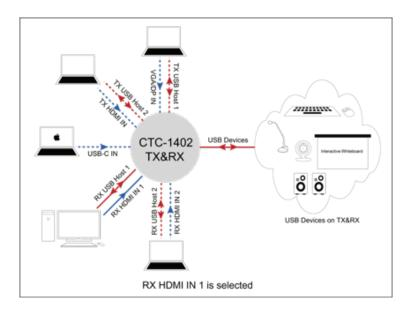
RX HDMI IN 1 and RX HOST 1 are in a group. Only if the RX HDMI IN1 is selected, the USB devices can be connected to the PC which is connected to RX USB HOST 1.
