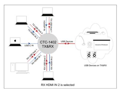
RX HDMI IN 2 and RX HOST 2 are in a group. Only if the RX HDMI IN 2 is selected, the USB devices can be connected to the PC which is connected to RX USB HOST 2.
