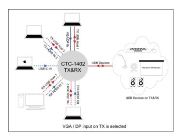
VGA IN 1, AUDIO IN 1 and HOST 1 are in a group, DP IN 2 and HOST 1 is in a group. Only if the VGA or DP is selected, the USB devices can be connected to the PC which is connected to USB HOST 1.
