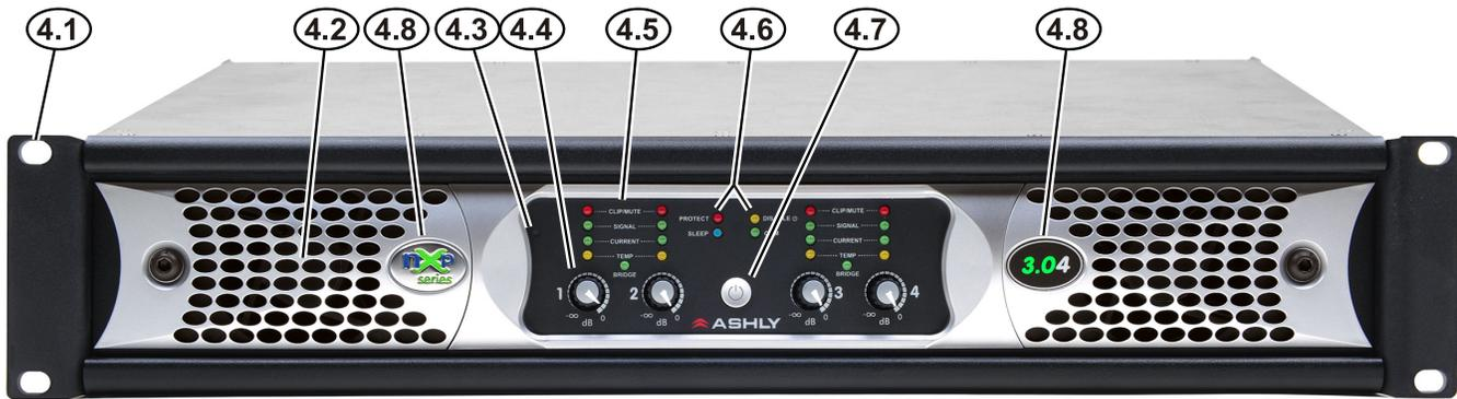
**4.1 Mounting Holes** – For mounting to a 19" equipment rack.
