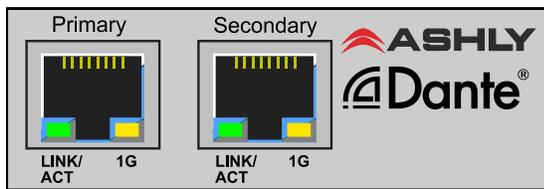
Dante, created by [Audinate](#), is an Ethernet based digital AV network technology that uses existing 100MB or 1GB network infrastructure for delivery of high performance, high channel count audio signals. Ashly products with network audio capability can
