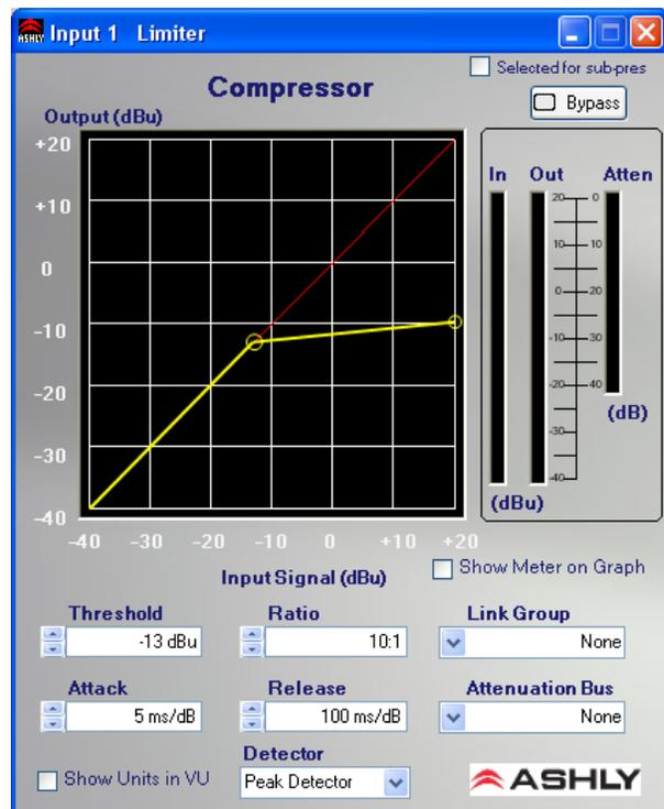
**Release Time** - The rate (in ms/dB) at which the Compressor attenuation will return to normal, once the signal falls below Threshold.
