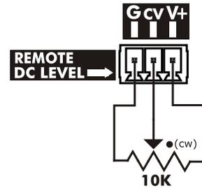
**5.3 Remote DC Level Control** - Each channel has a potentiometer circuit available for remote DC Level Control. The example to the right illustrates a typical DC level control application. There is no limit to wire length, but do not use any other ground source. If multiple remote DC level controls are used for different channels, the same ground and V+ sources can be shared.
