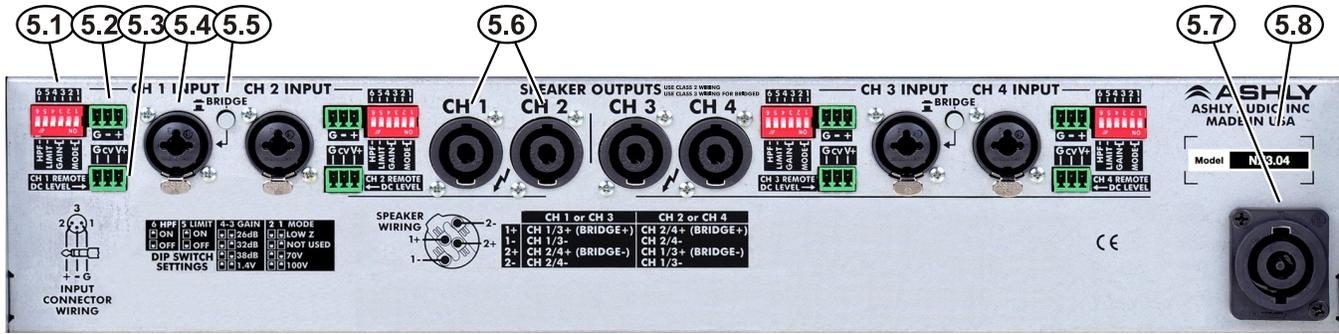
**5.1 Channel Configuration DIP Switch** - The DIP switches configure each channel's 80Hz 2nd Order Hipass Filter, Output Clip Limiter, Amplifier Gain, and Output Mode. In the example to the right, the DIP switch is set as follows: **6**: 80Hz High Pass Filter is Off; **5**: Clip Limiter is On; **4&3**: Gain is 1.4V; **2&1**: Output Mode is Low Z.
