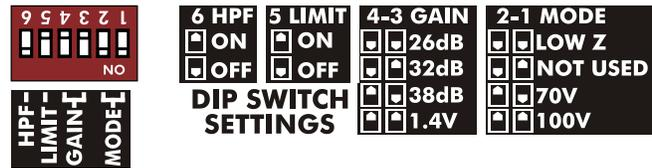
*Note: The Gain setting of 1.4V means that a 1.4V input will drive the amp to full output in any output mode. The other three Gain settings will apply their respective amplifier gain regardless of output mode, so the actual input voltage required to fully drive the amp will vary based on the selected output mode.*
