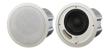
block that allows direct connection to the speaker with up to 2.5 mm (12 AWG) wire and provides pass through to additional speakers. Two adjustable metal tile bridges and metal "C" ring are included for safe suspension of the EVID PC6.2 ceiling systems in a drop ceiling that uses mineral wool, or other fiber-based ceiling tiles. The wide range of EVID ceiling speakers has been designed to work together as a complete system in a variety of different ceiling constructions.
