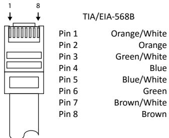
The TCP/IP port requires a standard straight-through Category 5 or greater cable with the TIA/EIA-568B crimp pattern for operation.
