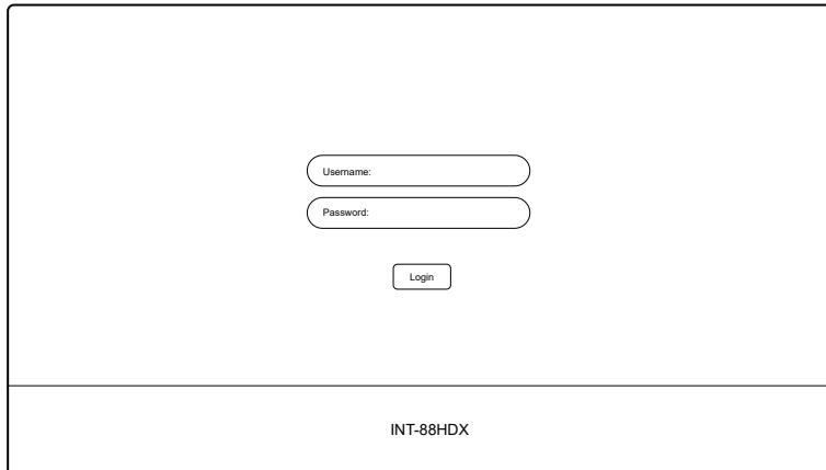
Open a web browser and go to the IP address of the INT-88HDX. The default IP address is 192.168.0.178.
