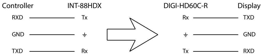
Insert the removable three-pole terminal block into the RS232 tunneling port for the output zone which requires remote RS232 control.
