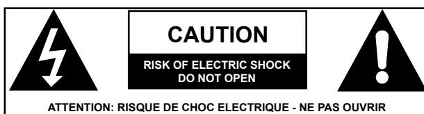
**!** 27. This lightning flash with arrowhead symbol within an equilateral triangle is intended to alert the user to the presence of non-insulated "dangerous voltage" within the product's enclosure that may be of sufficient magnitude to constitute a risk of electric shock.
