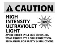
RISK GROUP 3 - RISK OF EXPOSURE TO ULTRAVIOLET UV RADIATION! FIXTURE EMITS HIGH INTENSITY WAVELENGTH OF ULTRAVIOLET UV LIGHT FROM THE UV LED. WEAR PROPER EYE AND SKIN PROTECTION. AVOID PROLONGED PERIODS OF EXPOSURE TO UV LED. AVOID WEARING WHITE COLOR CLOTHING AND/OR USING UV PAINTS ON SKIN.
