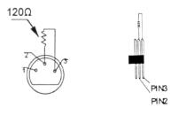
Termination reduces signal errors and avoids signal transmission problems and interference. It is always advisable to connect a DMX terminal, (Resistance 120 Ohm 1/4 W) between PIN 2 (DMX-) and PIN 3 (DMX +) of the last fixture.
