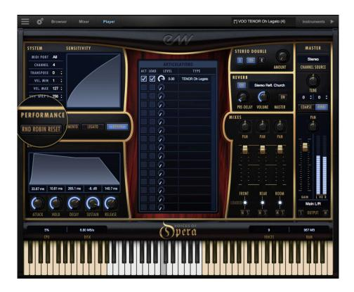
**Automatation:** Performance scripts can be automated by sending MIDI Continuous Controller (CC) values to the specified controller lane.
