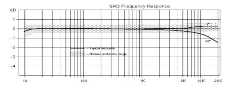
The SRO is a general purpose omni for live sound and recording. It handles huge SPL, has no proximity effect and no handling noise. It has fast clean impulse response and delivers accurate uncolored sound. Whereas, omnidirectional microphones are limited by feedback and leakage for many amplification applications, there are several types of applications for which they will deliver superior results.
