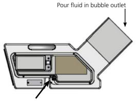
Fill to 0.5in below reservoir top. Do not overfill past top of reservoir.
