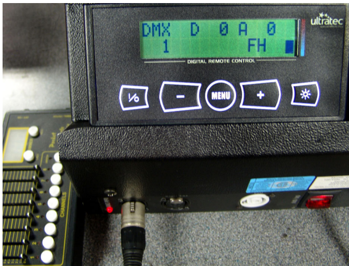
Machine warming up with DMX attached. Note "DMX" on screen with dmx address show below set at channel 1. Note valid DMX red LED now on (lower left).
