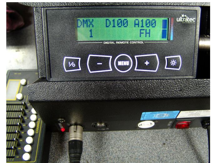
Machine on with DMX. Machine was fully heated (note bar graph) but heater starts for 100% Actual flow.
