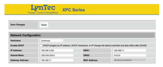
The Network Setup Page displays the current settings of the unit and the MAC address. This page is useful for retrieving all the information you may need to set up the XRS-80 on your network. Disable DCHP and set a static IP address for the XRS-80.
