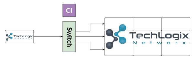
Encoder required: **one TL-IPFO-T01**Decoder required: **multiple TL-IPFO-R01**
