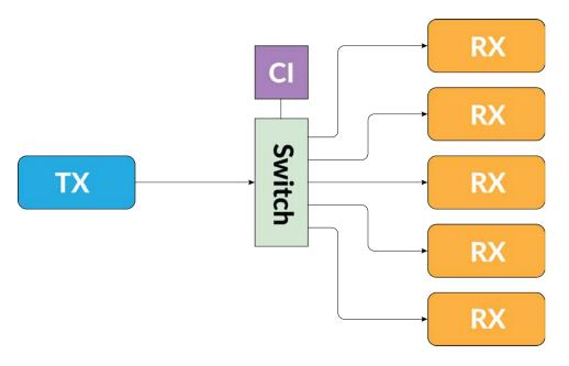
Encoder required: **one TL-IPFO-T01**Decoder required: **multiple TL-IPFO-R01**
