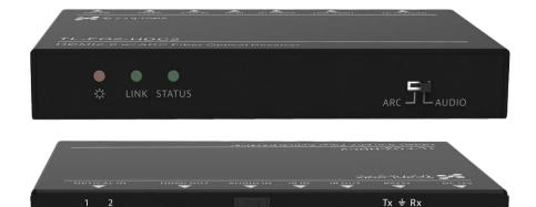
The TL-FO2-HDC2 is an HDMI 2.0 (18G signal) with HDCP 2.2 support fiber optic extender that can reach up to 300 meters (984 ft) over a duplex OM3 or OS2 cable with common LC terminations. The unit supports HDMI video resolutions up to 4K@60, HDR video, IR or RS232 pass-through controls, multichannel audio, as well as ARC with optional optical audio embedding and/or de-embedding. The TL-FO2-HDC2 is also compatible with HDMI 1.3/1.4 content with HDCP 1.3/1.4 content protection.
