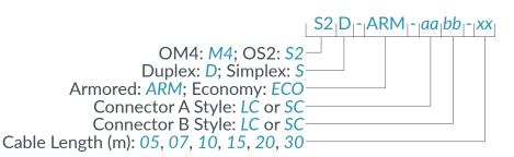
If an installation requires a 15 meter long cable with LC connectors on one end and SC connectors on the other, the part number to order is: S2D-ARM-LCSC-15.
