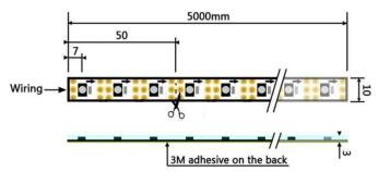
• 50mm spacing between each cutting point.
