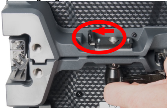
3. The vertical connector will snap into place when the latch snaps back to lock connector.
