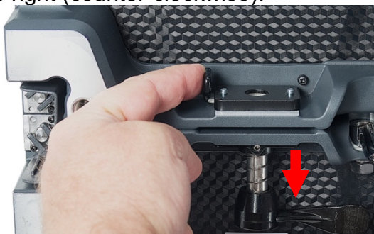
7. Once latch is released, the vertical connector will snap open.
