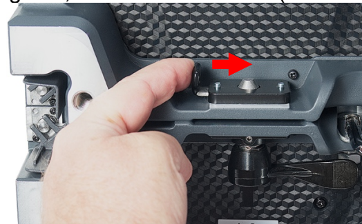
6. Press spring-loaded locking socket latch towards the right.
