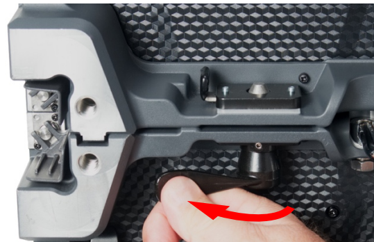
4. To tighten, twist lever to the left (clockwise).
