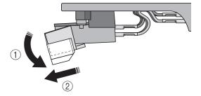
3 While using your fingers to hold the body of the cartridge, insert the tab of the replacement stylus into the groove on the underside of the cartridge.
