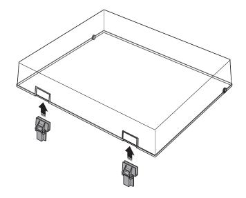
Attach the dust cover by inserting the hinges into the hinge bases located on the back panel of the unit.
