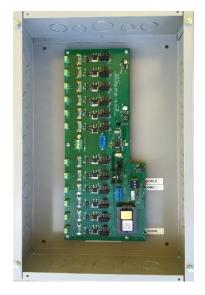
The DMX12DIM ELV-JBOX is a twelve output dimmer designed for high efficacy loads, and minimal losses. This dimmer uses "reverse phase" (aka: "trailing edge") dimming techniques and MOSFET power devices. This type of control is required for proper dimming of many LED fixtures. Each output can drive loads up to 100 Watts. Each channel may be configured for reverse phase dimming (default), forward phase dimming, or non-dim operation.
