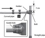
As a general rule, insert curved pipe until the guide hole on the pipe can be seen through the gap in the holder.
