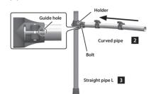
As a general rule, insert curved pipe until the guide hole on the pipe can be seen through the
