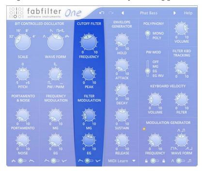
The **Frequency** knob adjusts the cut-off frequency. Basically, all sounds below the cut-off frequency will go through the filter, but sounds with higher frequencies are damped. At position 10, the cut-off frequency is far above 20 kHz and therefore the filter will allow all frequencies to go through unchanged. At position 0, the cut-off frequency is just a few Hz and the filter will block almost all sound from the oscillator.
