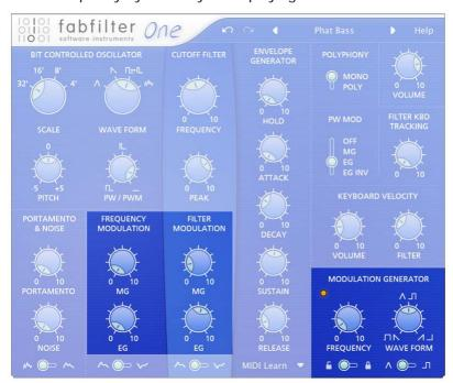
You can modulate the oscillator frequency and filter cut-off frequency with the modulation generator and the <u>envelope generator</u>. The filter cut-off frequency can also be modulated by velocity.
