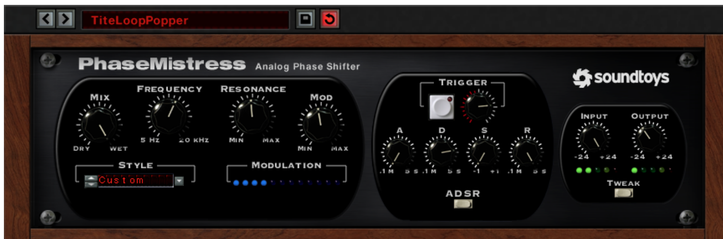
Figure 16: Control Panel layout in ADSR Mode
