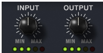
Figure 4: LED's indicating Input and Output signal level
