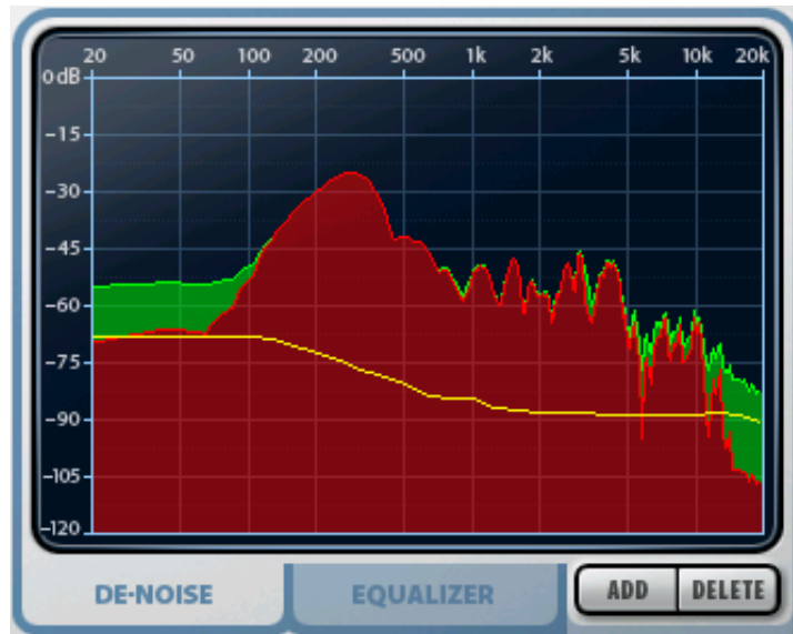
Figure 4-3. De-noise frequency display during processing. Mono display mode is selected.
