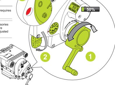
Hold and steady the camera, then disengage the tilt lock and observe how it moves and where it stops.
