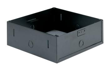
knockouts for conduit on four sides and slots for depth adjustment on two sides. It shall include welded torsion spring receptacles for installation of Lowell torsion grille Model FW-8T (ordered separately). The total weight of the speaker/transformer assembly used with the torsion grille shall not exceed 3.5 lbs.
