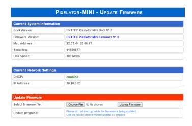
From this page you can update Pixelator Mini to the latest firmware. Latest firmware file is available at enttec.com/mini.
