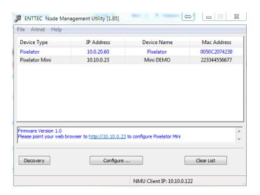
NMU (Node Management Utility) is a free Windows and Mac application that is used to manage compatible ENTTEC DMX over Ethernet nodes.
