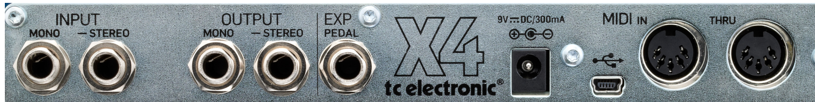
Flashback Triple Delay – rear
