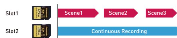
One SD card can be set in Slot 2 to record continuously, and another SD card can be set in Slot 1 to record necessary scenes by turning REC on and off.
