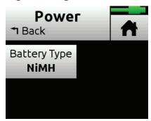
3. Select the type of batteries being used in the sled. Options include: NiMH, Alkaline, L-Mount
