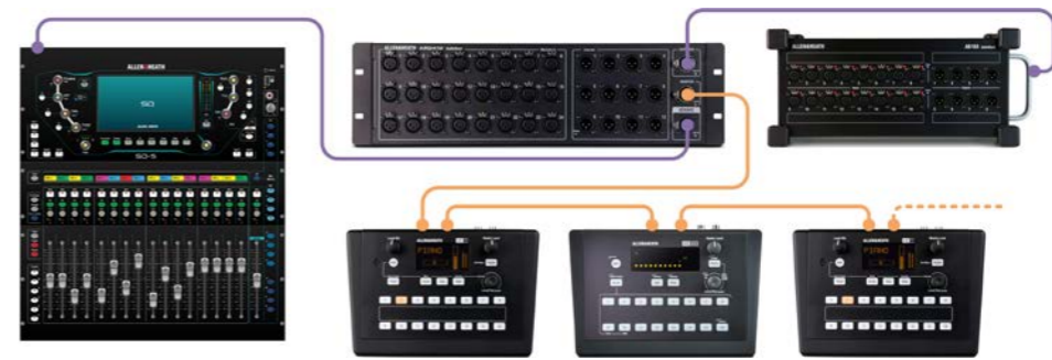
SQ expanded using AR2412 + AB168 40 remote inputs + 20 remote outputs + ME system
