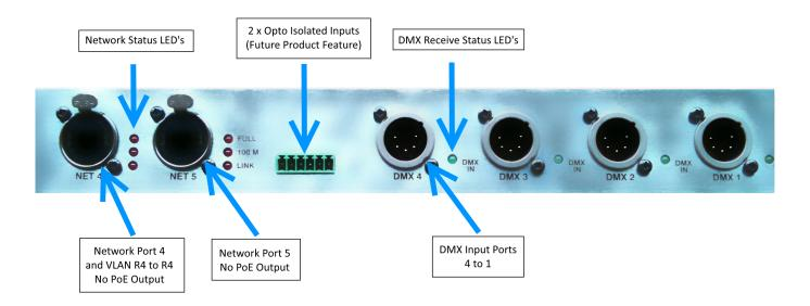
The two **NET** ports on the back of the device do not have PoE (Power over Ethernet) functionality. Both ports can be of general use, and **NET4** can also be used as the **VPN** link between two R4 units.
