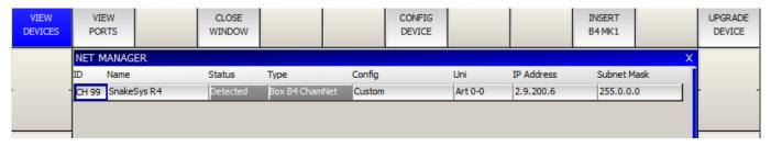
If you are sent a newer firmware file by ChamSys support then copy the file into the firmware folder in the MagicQ installation. To install it onto a MagicQ console put the file onto a USB stick, then in MagicQ go to Setup, File Manager. Select USB DRIVE. Press COPY and select the file as the soruce to copy. Then select the destination, by selecting HARD DRIVE, UP DIR, and select the firmare folder. Press the "." item to copy to. Then follow the procedure above.
