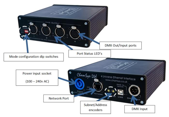
For simple Art-Net or ACN to DMX output conversion on the SnakeSys B4 the DIP switches/rotatory encoders can be used to quickly configure the device for this mode.
