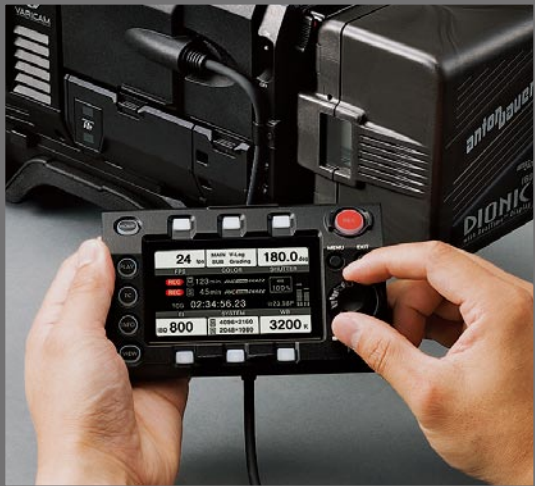
Detachable control panel
