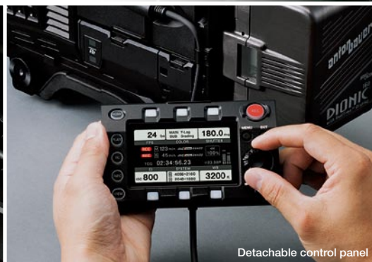
Detachable control panel
