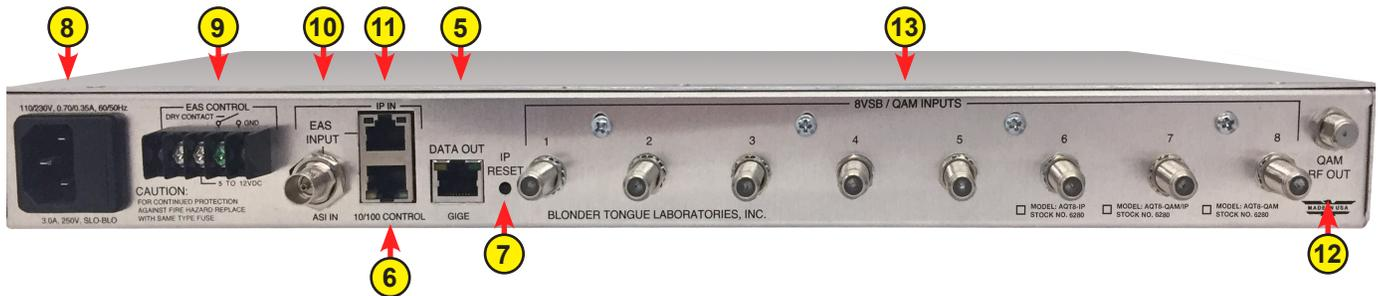
**8 INPUT POWER ASSEMBLY AND FUSE:** IEC 14 power inlet plug – rated 110-230 VAC; 0.7/0.35; 60/50 Hz; equipped with Slo-Blo, 3.0A, 250 V Fuse.
