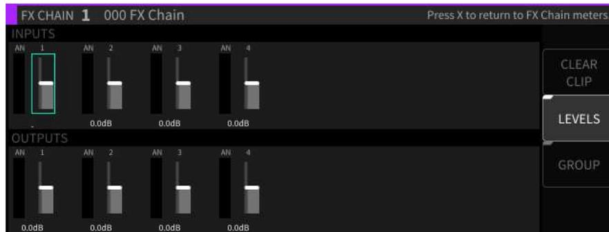
Use the cursor buttons to navigate to the input or output slider you wish to adjust, then use the wheel to adjust the signal level fader of the highlighted fader.
