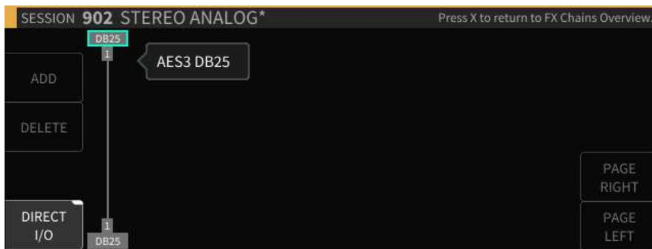
In the Direct I/O screen, use the cursor keys to highlight the input/output you wish to assign, then use the wheel to select the physical input /output you wish to use in your direct I/O pathway.
