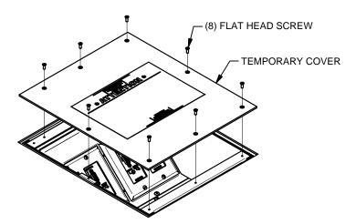
2. INSTALL CABLE INTERFACES AND CONNECTOR PLATES IF PREVIOUSLY NOT INSTALLED. CLEAN AREA IN AND AROUND ENTIRE TOP EDGE OF BOX AND APPLY 1/4" CONTINUOUS BEAD OF RTV SILICONE SEALANT.
