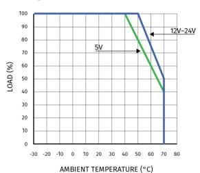
Recommended to reduce device load if running at high temperatures to prolong lifetime
