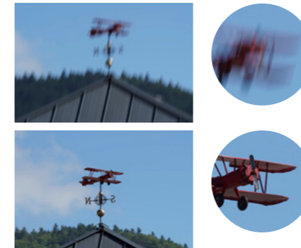
Compensation for commonly experienced pitch and yaw shake at long focal length shown at bottom.
