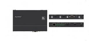
The DIP-31 is a 4K@60Hz (4:2:0) automatic switcher for HDMI, VGA, Ethernet, data and unbalanced audio signals. It supports various modes of input selection and transmit the signal via HDMI cable to a compatible receiver (for example the VS-62H or a display/projector). The device is a Step-in commander when connected to a matrix switcher that supports Step-in over HDMI such as the VS-62H. It also features RS-232 commands to support monitor/projector on/off
