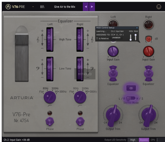
V76-Pre ready for MIDI learning. Notice the MIDI control setup window over the selected control, which is already assigned (when assigned, the color changes to red).
