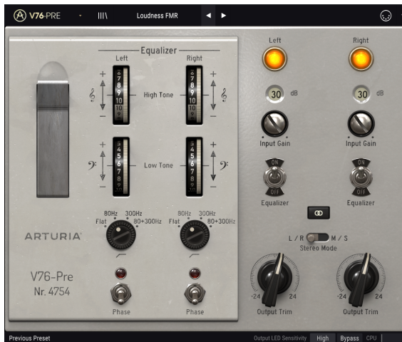
V76-Pre configured to add some 'loudness' to the sound. The High Pass filter is also switched to cut frequencies below 80Hz
