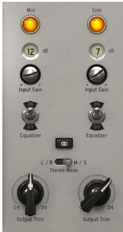
V76-Pre Double Channel Preamp and Output. Notice the Stereo Link and Stereo Mode switches, right above the Output Trim controls, and the Glowing Output Lamps on top
