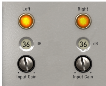
V76-Pre Double Channel Glowing Output Lamps and Preamp gain controls
