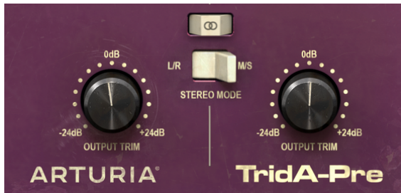
The lower right section of the TridA control panel, showing the Output Trim knobs, and above them the two switches that control the behavior of the plug-in in Double Channel: the Stereo Mode and the Stereo Link.
