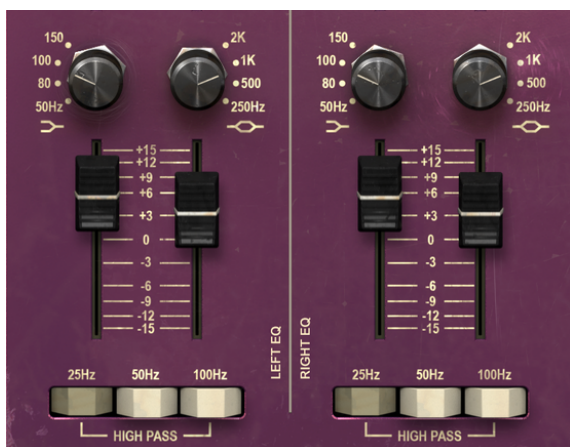
TridA Double Channel EQ lower bands (Low Shelf and Low Midrange Bell), and the three High Pass Filter switches on the bottom
