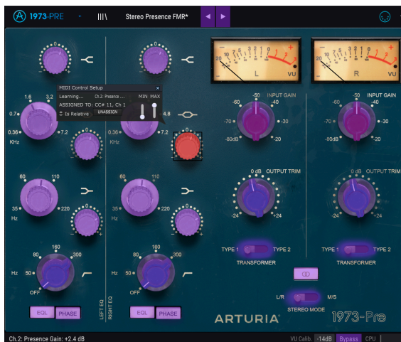
1973-Pre ready for MIDI learning. Notice the MIDI control setup window over the selected control, which is already assigned (when assigned, the color changes to red).
