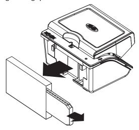
**2** Remove the enclosure lid by pushing out and lifting up.
