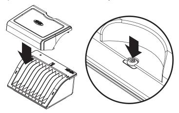
6 Secure the enclosure unit to a desk using the included combination cable lock.
