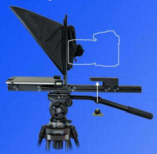
It is important that the camera lens is in the centre of the aperture at the rear of the hood. This is achieved by raising and lowering the hood and fitting a camera riser.
