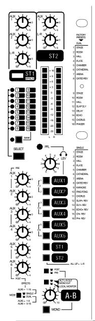
The WZ12:2DX and WZ16:2DX are provided with a built-in stereo digital effects processor. This can be configured as a single dual stereo effect (eg reverb + echo) fed from aux 5 or as two independent stereo effects fed respectively from aux 5 and aux 6.
