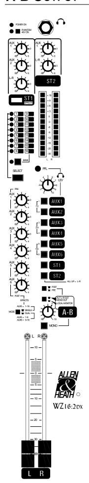
The A-B output is an additional stereo/mono output that can be uniquely configured as either a **separately controllable mix** output, or a **local loudspeaker monitor** feed.
