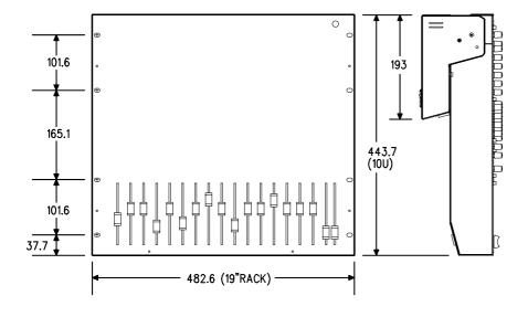
Mount the console in the rack using 4x M6 bolts each side for maximum strength. We recommend you fit the bolts with plastic cup washers to protect the panel, and they look good... These should be available from the supplier of the rack unit or a good hardware store.
