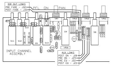
channel assembly allow pre-EQ and/or pre-ON if required. This is shown in the diagram below. **CHANNEL DIRECT OUTPUT SOURCE**
