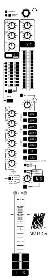
Two stereo return inputs **ST1** and **ST2** are provided giving you a total of 20 inputs to the L-R mix on the WZ16:2DX, or 16 inputs on the WZ12:2DX. These may be used for returning the processed signal from the effects devices, monitoring and replaying your 2-track recording, expander or submix inputs, or for stereo intermission replay.
