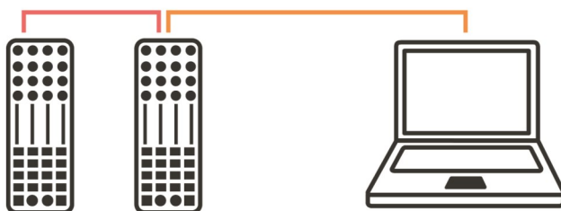
K1 CONTROLLERS via X:LINK + LAPTOP via USB
