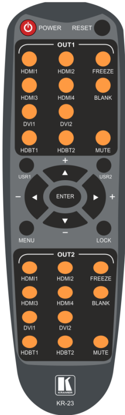
Figure 27: Infrared Remote Control Transmitter
