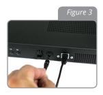
Connect the power cable to the AE server. Use only the 5V DC power supply provided with the server. Use of other power supplies may cause damage to the server.
