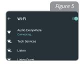
Connect the smart phone or tablet to the Wi-Fi network. Make sure that the AE server and smart device are connected to the same Wi-Fi network.
