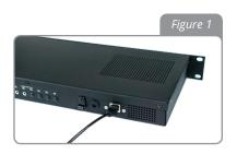
Connect the AE server to the local area network (LAN) via the ethernet port on the back of the server. The LAN should have at least one wireless access point (WAP) and a router, wireless router or a DHCP server. An ethernet cable has not been provided to make this connection.
