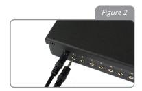
Connect the audio sources to the AE server. This requires a 3.5mm stereo jack connection to the server. One sixfoot cable has been provided for each channel. Custom cables with 3.5mm male stereo jacks may be used as well.
