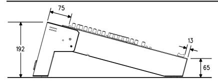
The console is fitted with rubber feet to ensure it does not slip or scratch the work surface. The control panel is angled at 15 degrees for operating convenience.
