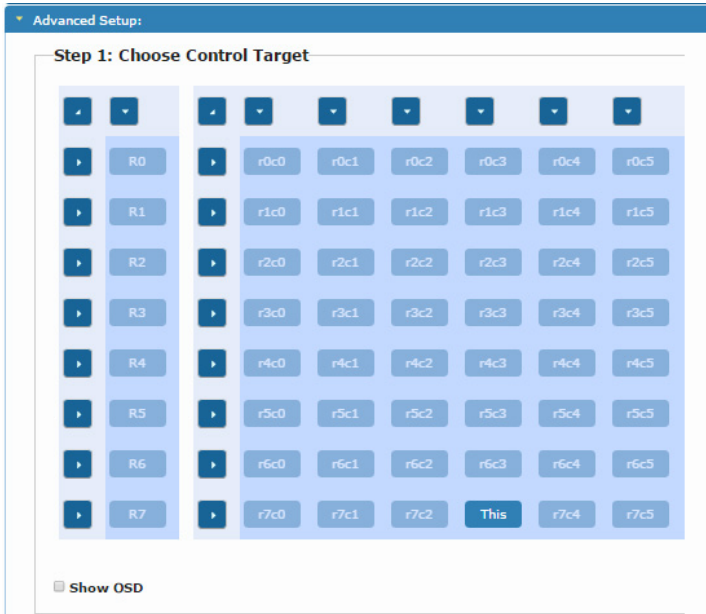
Figure 20: Video Wall Tab – Advanced Setup, Selecting a specific Device, Column or Row
